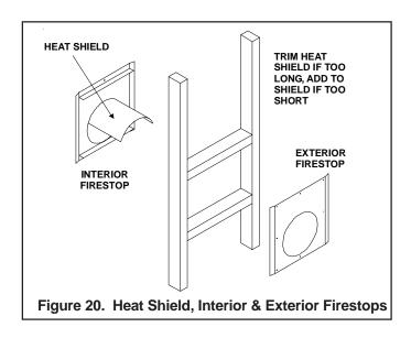
**For Vertical Runs -** One ceiling firestop is **REQUIRED** at the hole in each ceiling through which the flue passes.
